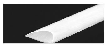
Figure 28. Skew chisel.
